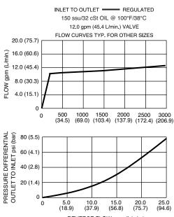
REVERSE FLOW gpm (L/min.) (24 GPM valve with control orifice)
